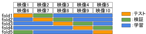
図5 k-分割交差検証(k=5) Fig.5 k-fold cross-validation.
